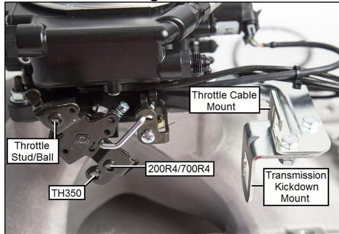
3. Reconnect the throttle and transmission kick-down linkage. Be sure to check for any binding conditions and correct before proceeding.
